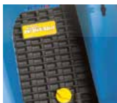
Glove compartment with handy access to check pump oil level
